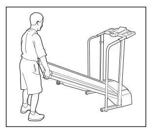
2. Move your right hand to the position shown and hold the treadmill firmly. Raise the treadmill until the storage latch closes over the catch. Make sure that the storage latch is fully engaged over the catch.
